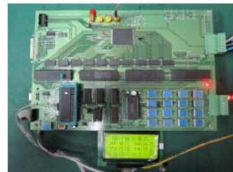
Fig.2 Circuit board of trigger generator 图 2 脉冲发生器实物图
