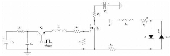
Fig.3 Main circuit of the driver 图 3 驱动电路原理图
