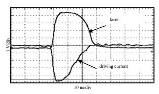
Fig.6 Drive current and output laser pulse waveforms 图 6 驱动电流与输出激光脉冲波形
