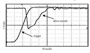
Fig.7 Drive current and trigger pulse waveforms 图 7 驱动电流与触发脉冲波形
