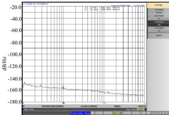
Fig.4 Phase noise test results of the 80 MHz crystal oscillator
