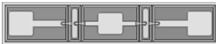
Fig.3 TeraTech GaAs anti-series Schottky diodes 图 3 TeraTech GaAs 反向串联肖特基二极管
