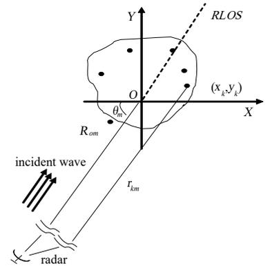
Fig.1 Relative geometric relationship between target and radar
