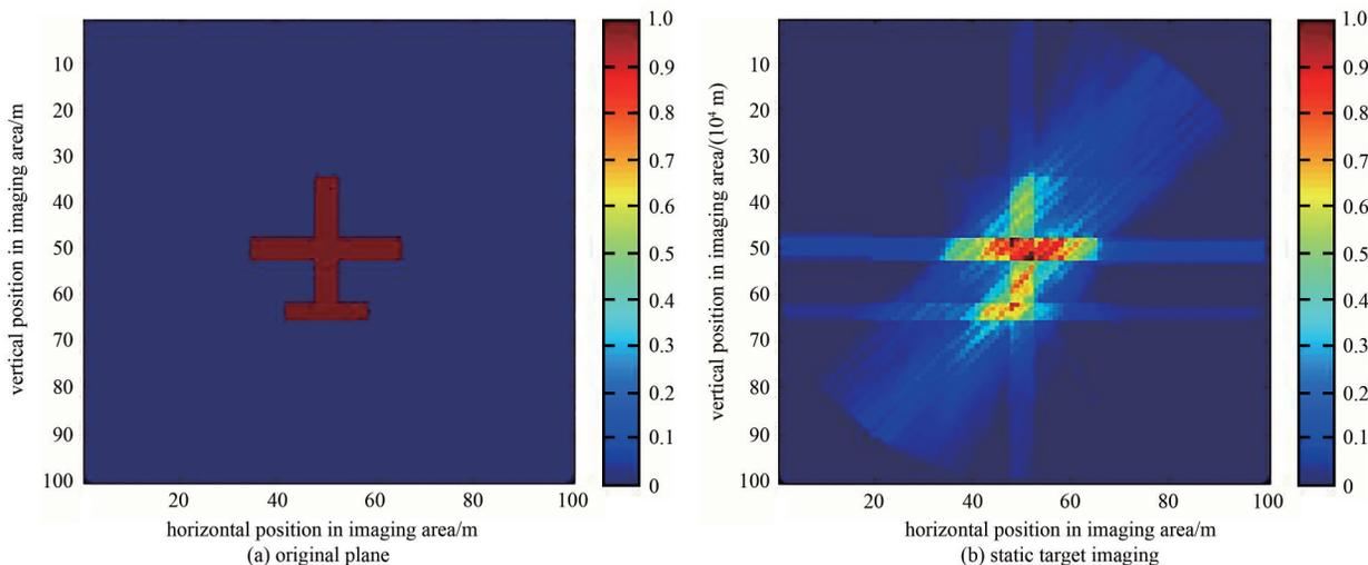
Fig.4 Imaging effect of static radar target
