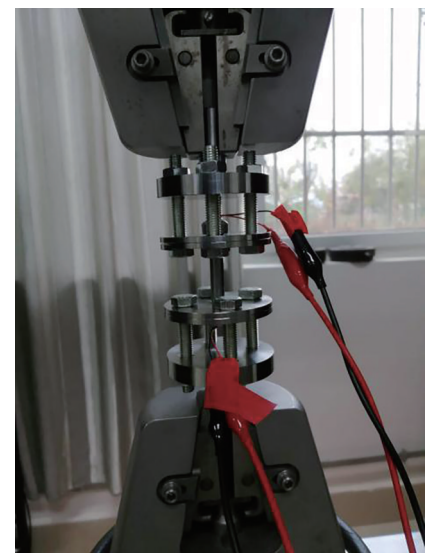
Fig.6 Force loading device of acoustic elasticity test
