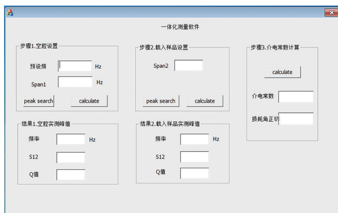
Fig.5 Interface of integrated permittivity measurement software
