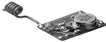
Fig.3 Contour of 433/868 MHz receiver
