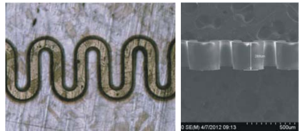
(a) optical microscope picture (b) SEM picture Fig.8 SU8 models exposed by 200 s 图 8 曝光量为 200 s 时的胶膜图形
