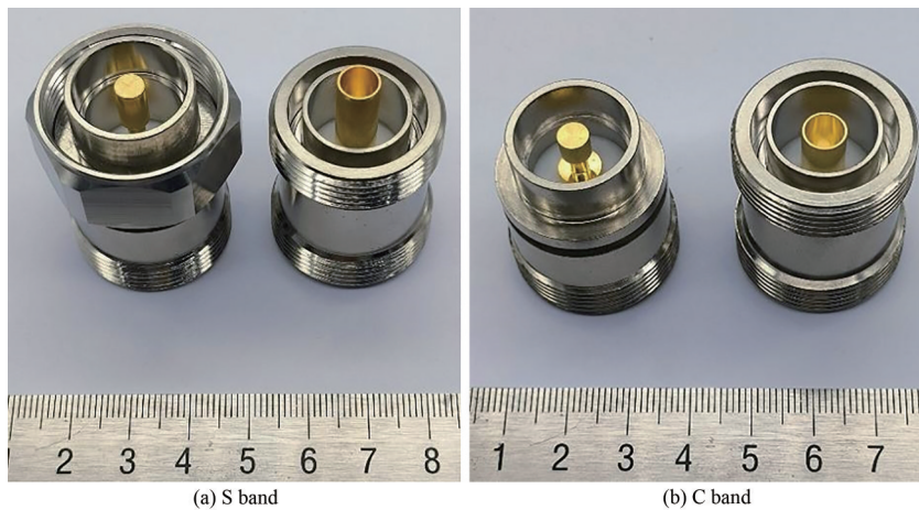
Fig.5 Pictures of the contactless coaxial connector of the inner conductor at S band and C band
