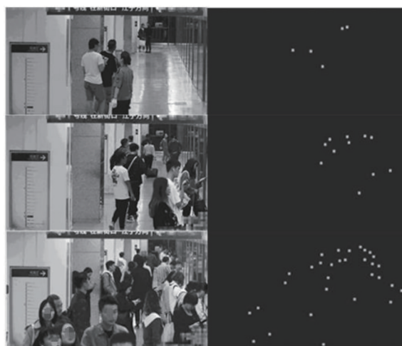
Fig.3 Convert label image to density map 图3 标注图转成密度图
