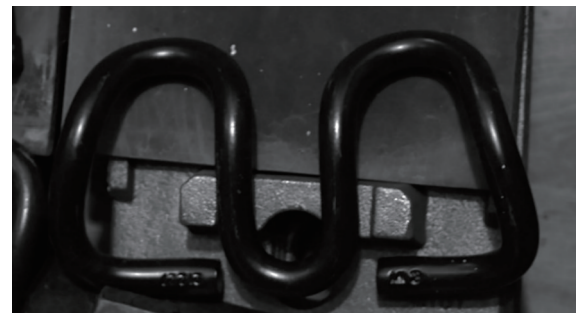
Fig.8 Typical defective fastener images clip
